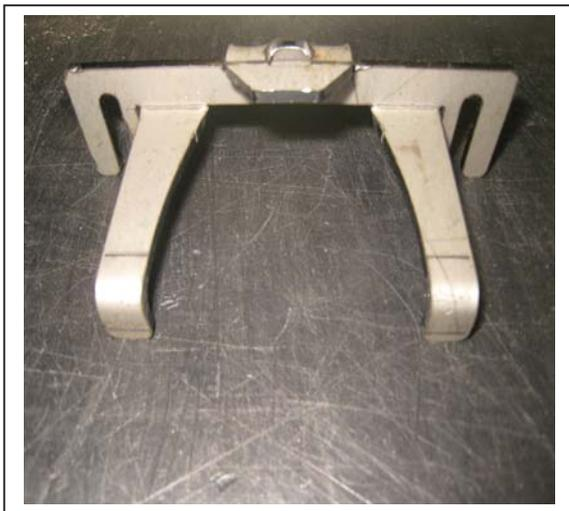
FIG 1 Shipping Clip to secure hopper
