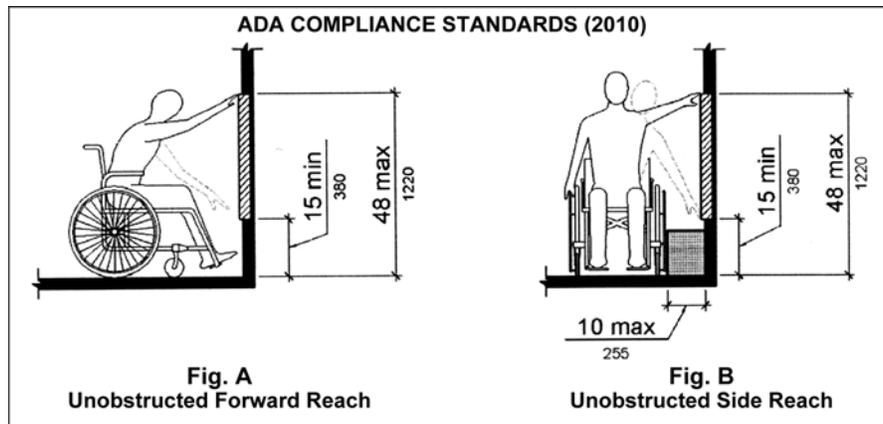
Below is a chart listing each MC cabinet model and the corresponding **MAX INSTALLATION HEIGHT** necessary to comply with the ADA requirements. The measurement shown is taken from the base (bottom) of the machine to the floor. Additionally, ADA requires a 30” (760mm) by 48” (1220mm) “clear floor space” to provide sufficient clearance for a single wheelchair and occupant.
