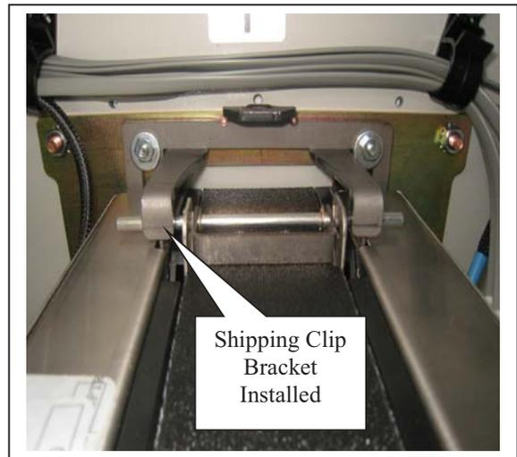
FIG 2 Shipping Clip Installed at top
