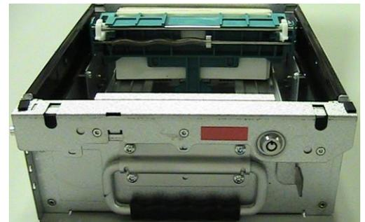
**STEP 3** – Pull the green pressure plate towards you and insert a stack of good conditioned bills.
