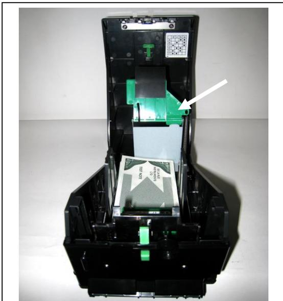
**STEP 3** – Lift pressure plate in rear as shown.
