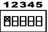
1. Activate the Overpay Timer programming mode by setting: Switch 1-ON; Switch 2-OFF; Switch 3-OFF; Switch 4-ON; Switch 5-ON
