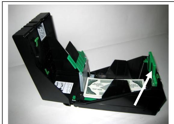
**STEP 4** – Lift pressure plate in front and load bills.
