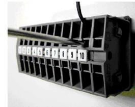
**IMPORTANT** ó Check all spring loaded terminal block and PLC screw connections before testing the GXP and wash bay. Gently pull on the wires to make sure they are secure.
