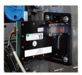
**Bi-Directional, Weatherproof Card Reader reads the mag stripe from either direction**, and is angle mounted to allow coins to fall out when inadvertently inserted. (Credit Card Acceptance Optional)
