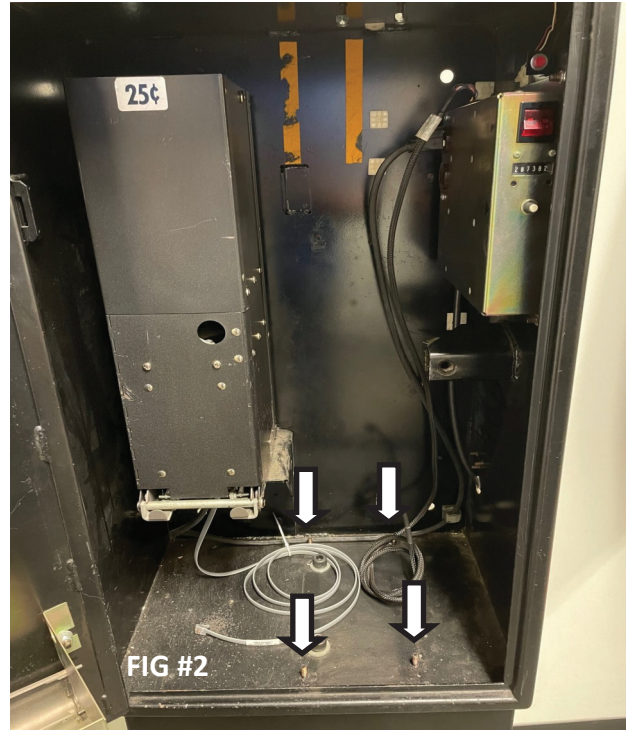
System 200/A Validator removed from the cabinet. Arrows show locations of the Mounting Studs for the SC Controller Tower (same studs used by the System 200/A validator)
