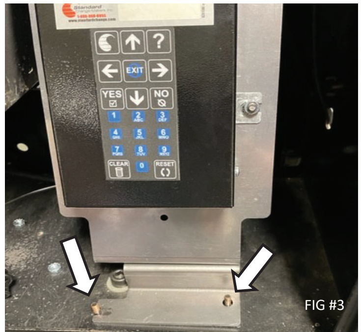
System 200/A Validator removed from the cabinet. Arrows show locations of the Mounting Studs for the SC Controller Tower (same studs used by the System 200/A validator)
