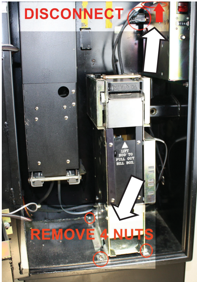
System 200/A Validator removed from the cabinet. Arrows show locations of the Mounting Studs for the SC Controller Tower (same studs used by the System 200/A validator)
