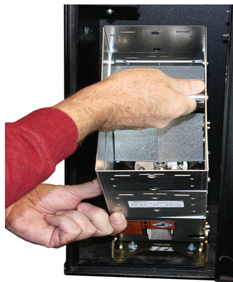
MC POWER SUPPLY INSTALLED ON THE SAME MOUNTING STUDS ON BACK WALL
