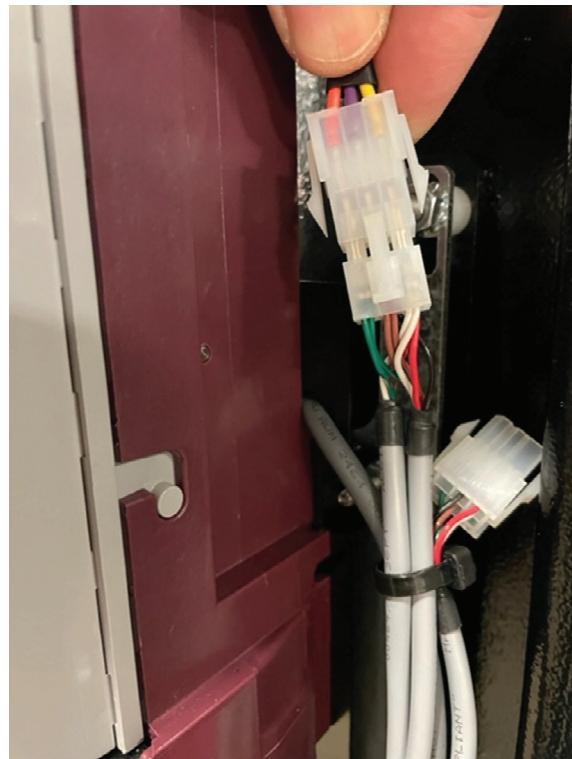
Connecting to a new Pyramid APEX-7000 or CPI T7 Talos Series acceptor
